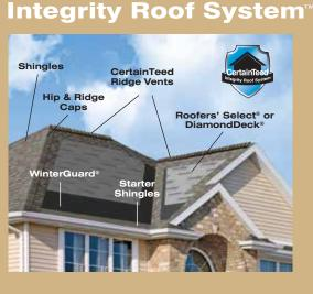
A systems approach combines highperformance components - underlayments, shingles, accessory products and ventilation - to make the Integrity Roof System a complete roofing solution. When you choose an Integrity Roof System, you gain the advantage of having CertainTeed as your single manufacturing source to stand behind its roof system components.
